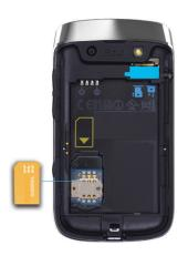
Slide the SIM card into the slot.
